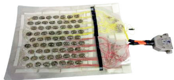
FIGURE 2. Prototypes of the flexible electrode: (A) device with diameter 8 cm with hexagonal electrode disposition, (B) removable needles inserted in electrical connection and (C) square device 15 x 15 cm with hexagonal arrangement of conductive guides highlighted.
