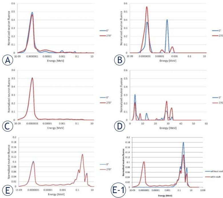
**FIGURE 2.** Neutron spectra in measuring positions (A), (B), (C), (D) and (E) for photon field size 10 x 10 cm<sup>2</sup> and gantry angles 0° and 270°. (E - 1) is normalized neutron spectrum in measuring position E for simulations with and without vault.
