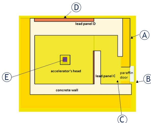
**FIGURE 1.** Top view (down) of the vault where Siemens Oncor Expression accelerator at Osijek University Hospital is placed with marked positions of measurements. (A), (B) and (D) are positions outside the vault, (C) and (E) are inside the vault. Position E is in isocenter.
