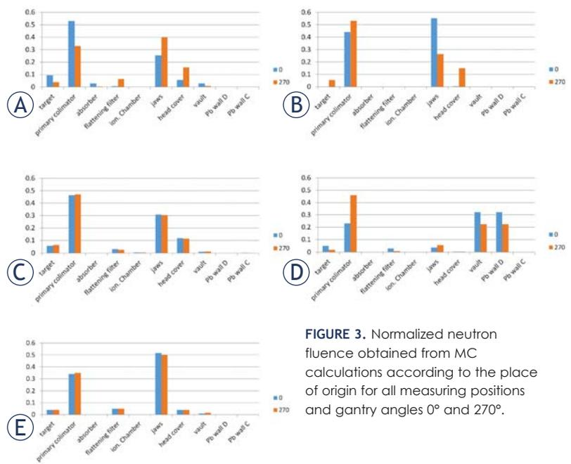
FIGURE 3. Normalized neutron fluence obtained from MC calculations according to the place of origin for all measuring positions and gantry angles 0° and 270°.
